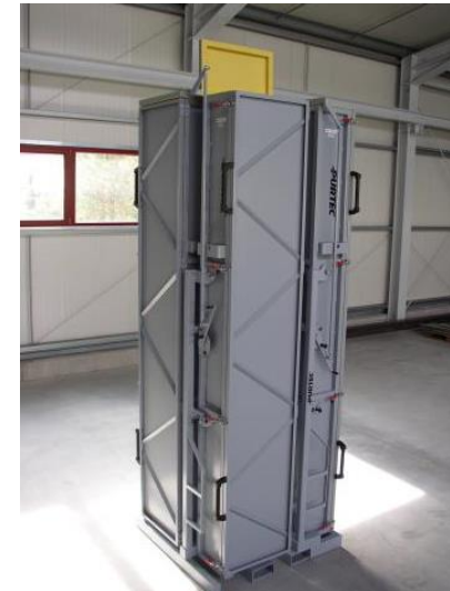
Steel frame with 4 intermediate storage and transport boxes 带有4个中间存储和输送箱的钢架
